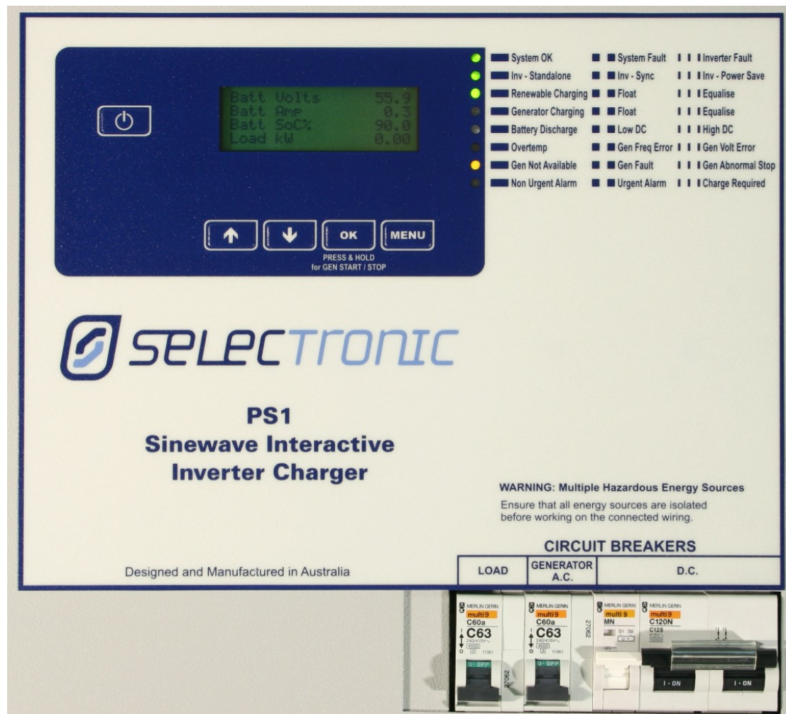
Figure 5 PS1 Circuit Breakers
