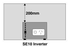
Please leave a clearance of 200mm on all sides and top of the Inverter. The SE10 must be installed in a dry, cool, dust-free environment. It is recommended that the inverter be placed as far from any radio receivers as possible.
