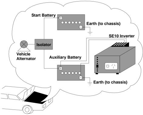
By incorporating an auxiliary battery in the manner above, the starting battery should remain charged for vehicle starting (see your auto electrician). The SE10 has sufficient battery cable length to allow it to sit underneath the vehicle whilst in use. If the ground is wet, place the SE10 on a waterproof liner.
