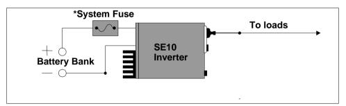
\* A system fuse (of at least 15 Amps) should be placed before the battery. An HRC motor start type is recommended. (See your system designer for details).
