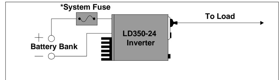
\* A system fuse (of at least 20 Amps) should be placed before the battery. An HRC motor start type is recommended. (See your system designer for details).
