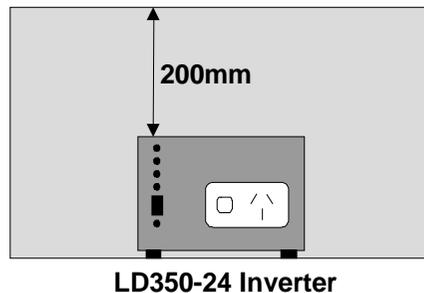
Please leave a clearance of 200mm on all sides and top of the Inverter. The LD350-24 must be installed in a dry, cool, dust-free environment. It is recommended that the inverter be placed as far from any radio receivers as possible.
