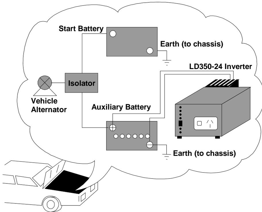
By incorporating an auxiliary battery in the manner above, the starting battery should remain charged for vehicle starting (see your auto electrician). The LD350-24 has sufficient battery cable length to allow it to sit underneath the vehicle whilst in use. If the ground is wet, place the LD350-24 on a waterproof liner.
